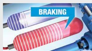
PowerBoost uses its pressure cells to capture wasted energy, which is used to power the vehicle.
